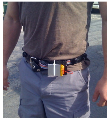
Haptic belt: Direction sense
